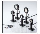
roughly the 10 kHz level. So if you are using a pulsed laser with a repetition rate less than 10 kHz you have a choice between measuring pulse energy with a pyroelectric sensor or average power with a thermopile sensor. Lasers with repetition rates faster
