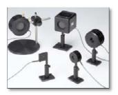
for many lasers. They are used for measuring CW laser power, average power in pulsed lasers, and are often used to integrate the energy of long pulses. Thermopile sensors absorb incident laser radiation and convert it into heat. This heat ultimately
